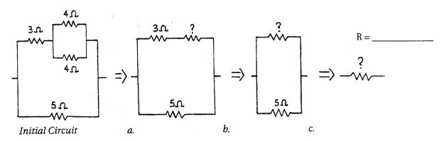
2. The circuit below is similar to Figure 35.11 in your textbook. In three successive steps, as in Question 1, replace each pair of resistors by a single resistor of equivalent resistance.
